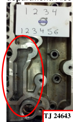
Photo 2. Intake side of PCV diaphragm
